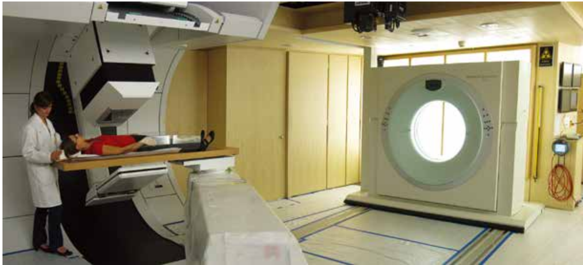
Figure 3 Photograph of Gantry 2 treatment room with gantry-angle set to +20^\circ . Visible on the left are the patient-table, the false fixed floor around the patient-table for easy access to the patient, the extractable nozzle, the rolling cover where the nozzle rotates and the BEV. Note that the BEV is extracted with the imager positioned along the proton beam direction just downstream from the patient. Noteworthy on the right is the sliding-CT, with the rails clearly visible on the floor. A white protective film is currently covering the floor and patient-table prior to treatment of first patient
