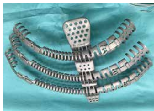
Figure 12 Titanium 3D printed implant with biomechanical design.
